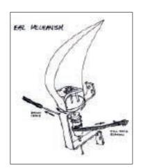
to move through at least 180 degrees, pointing forward they show interest, pointing backwards they indicate fear or alarm, and to the side they show attentiveness. The solution came to me early one morning: mount the ears on short vertical axles, around which would be wound a cable, with a spring to pull the axle back into place and rewind the string. The pull through 90 degrees, but the shorter circumference of the axle would give double that for the ear.
