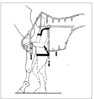
The puppeteer 'breathes' for the horse by bending his legs. The front legs rest on the ground whilst the chest is operated by the backpack attached to the puppeteer's shoulders and trunk. The front leg axle moves in a slot mounted on the horse's body frame © Adrian Kohle
